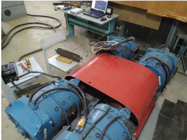
Fig. 1. External view of the test bench for investigating a series-excited DC traction motor operating in generator mode
